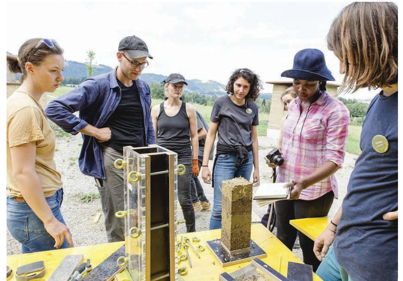
Participants experiment with Rammed Earth during a workshop at the BASEhabitat International Summer School in Altmünster, Austria (2018).
